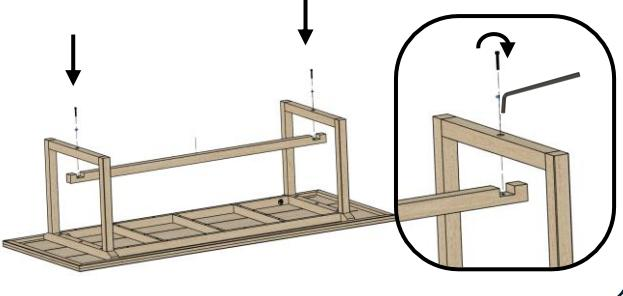
Attach the bottom rail to the legs by using the hex key to turn M8 bolts into the rail's bushings.
