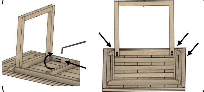
Use the provided bolts and hex key to tighten the legs in place.
