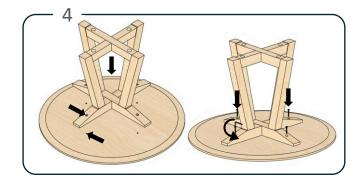
Place table top upside down and flip the frame so the holes in the top rails align with the pre-installed fittings in the top. Insert the bolts with washers and tighten using the hex key provided.
