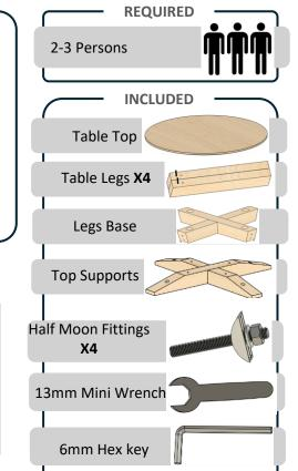
Insert the threaded rods into the pre-installed fittings of the legs. Position the legs at each end of the small cross and insert the rods into the pre-drilled holes. Insert the halfmoon washers and nuts onto rods and tighten using mini wrench.
