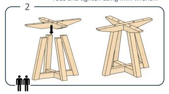
Position the big cross so the holes align with the preinstalled fittings on top of the legs.
