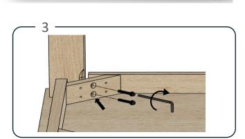
Use the Allen key with to fix the legs to the frame by turning the bolts with washers into the pre-drilled holes in the corner blocks.
