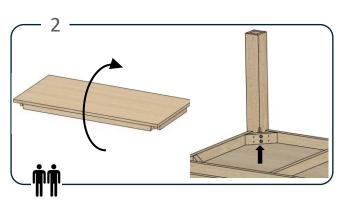
Turn the table top upside down and place legs in corners so that the holes align with the corner blocks.
