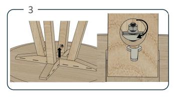
Insert the half moon washer and nut onto the threaded rod visible through the hole at the top of the leg.
