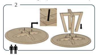
Turn the table top upside down and insert the wood dowels an threaded rods into pre-drilled holes.
