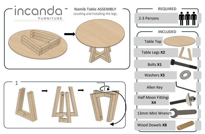
Remove the legs and slide the 2 parts into position where the cut-out joints connect. Turn the legs upside down and tighten the 2 parts using the provided bolt and hex key.
