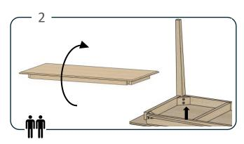
Turn the table top upside down and place legs in corners so that the holes align with the corner blocks.
