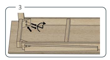
Use the Allen key with to fix the legs to the frame by turning the bolts with washers into the pre-drilled holes in the corner blocks.
